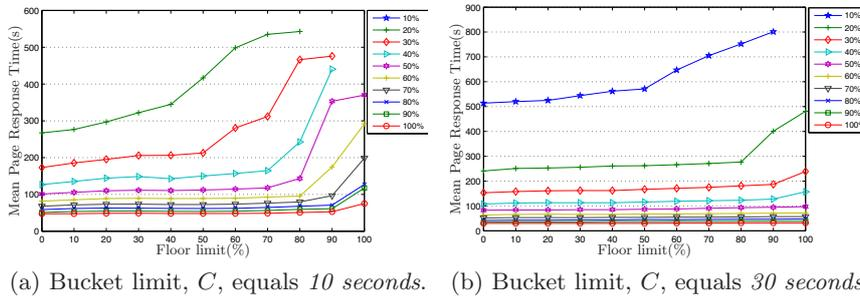
Fig. 4: Mean page response time of the browsing application for various levels of the traffic contract as function of the floor limit  $F$ . There is *one user* that makes use of the traffic contract.
