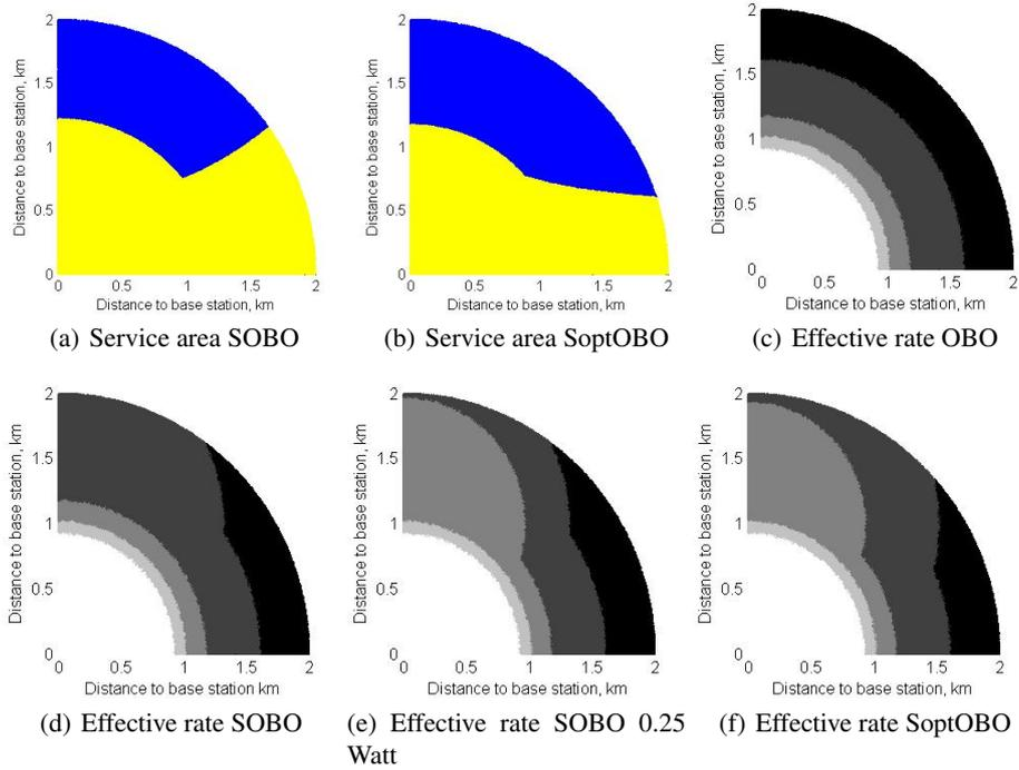
**Fig. 5.** Spatial behaviour in the cell with a relay station located at 1 km and transmit power 0.125 Watt. Shape of service area for: (a) SOBO and (b) SoptOBO. Effective data rates for: (c) OBO; (d) SOBO; (e) SOBO with RS transmit power 0.25 Watt; and (f) SoptOBO.
