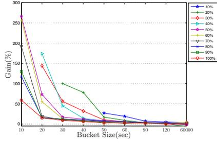
Fig. 5: The gain in response time as a function of the bucket limit  $C$ . The gain is expressed as the ratio of the mean page response time of the discussed policing solution divided by the mean page response time for the traditional leaky bucket policing mechanism with *one user*.
