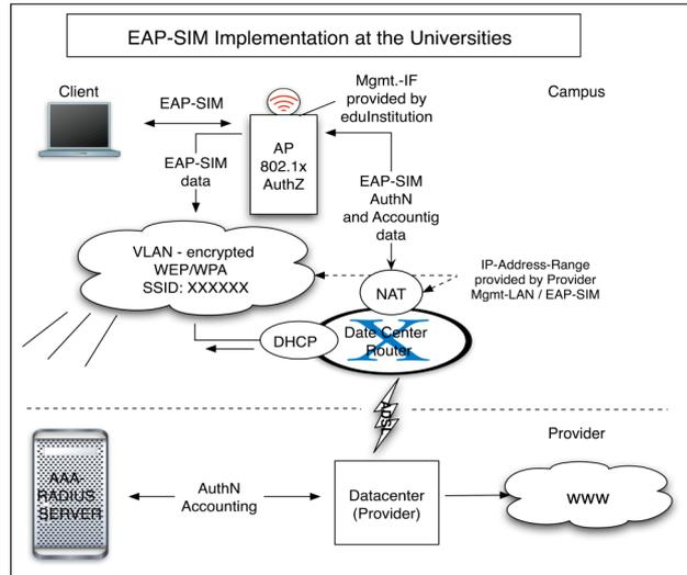
**Fig. 1.** EAP-SIM Extension Architecture at each University
