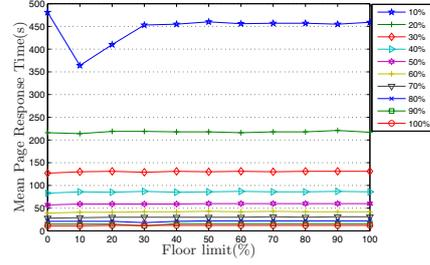
Fig. 6: Mean page response time of the browsing application for various levels of the traffic contract as function of the floor limit  $F$ . There are *five users* that make use of the traffic contract and the bucket limit,  $C$ , equals *30 seconds*.
