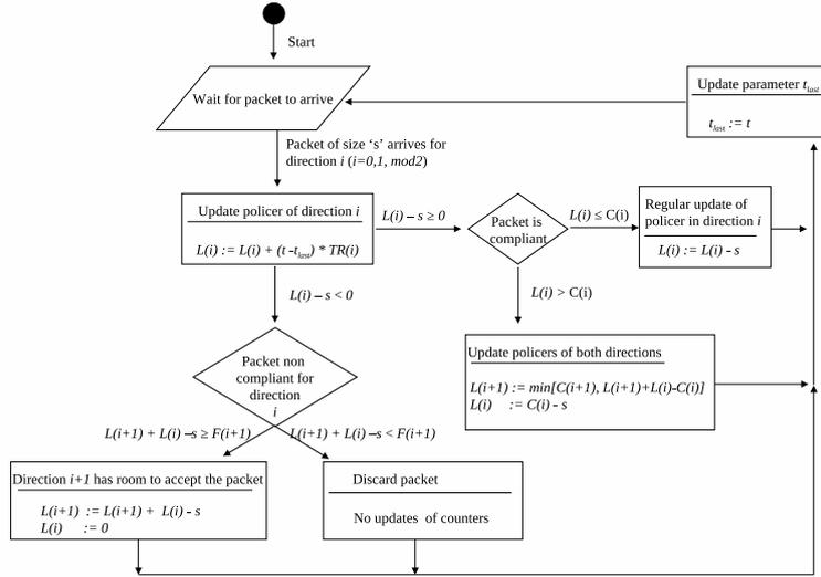
Fig. 1: State diagram for policing in two directions concurrently and preventing starvation in one of the directions. Here the parameters  $L(i)$ ,  $C(i)$ ,  $F(i)$ ,  $TR(i)$  denote respectively the bucket level, the ceil bucket limit, the floor bucket limit, and the token rate in direction  $i$  ( $i = 0, 1, \bmod 2$ ).
