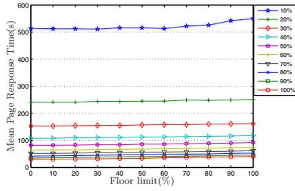
Fig. 7: Mean page response time of the browsing application for various levels of the traffic contract as function of the floor limit  $F$ . There is *one user* that makes use of the traffic contract and the bucket limit,  $C$ , equals *30 seconds*.
