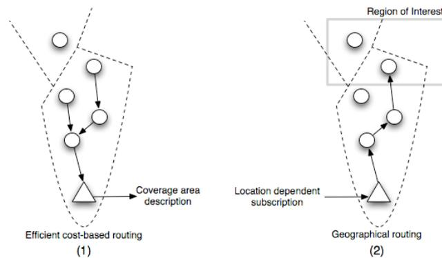
**Figure 1:** The WSN provides coverage area description to gateways (1) and reuse of collected information to route location dependent subscriptions (2)
