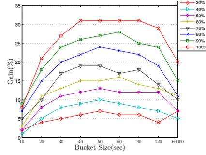
Fig. 8: The gain, expressed the ratio of the mean page response time of the discussed policing solution divided by the mean page response time for the traditional leaky bucket policing mechanism with *one user*.
