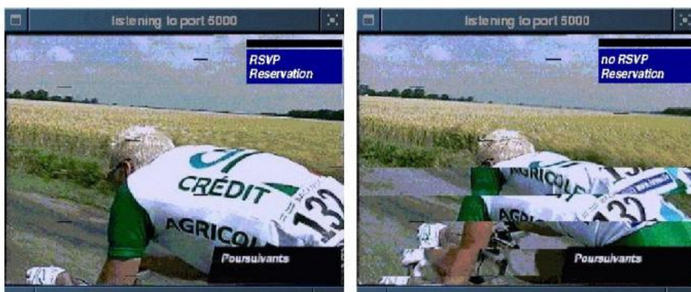
Figure 5.8: motion jpeg video transmission with and without bandwidth reservation. The picture errors occur from dropped UDP packets
