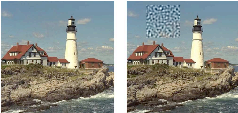
Figure 2.4: PSNR error examples: both images have the same PSNR. (Source [Winkler and Mohandas, 2008])
