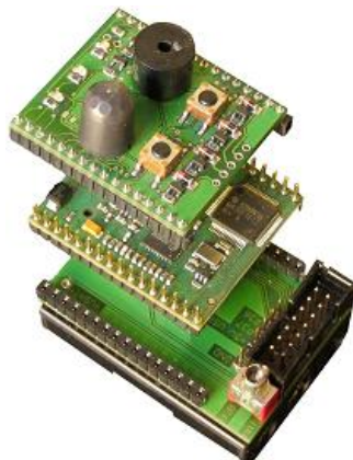
Figure 2.2: MSB430 Sensor Node Platform with pluggable Sensor Modules
