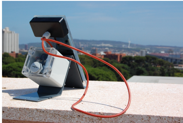
Figure 2: iSense node with Environmental and Solar Modules on a UPC building roof
