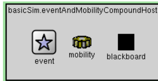
Figure 3.3: Inside the compound module EventAndMobilityCompoundHost , used to simulate moving objects. It includes the simple modules BasicEvent , Mobility and Blackboard
