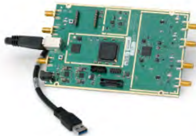
Figure 5.2: A USRP B210 device for Software Defined Radio reception [9].
